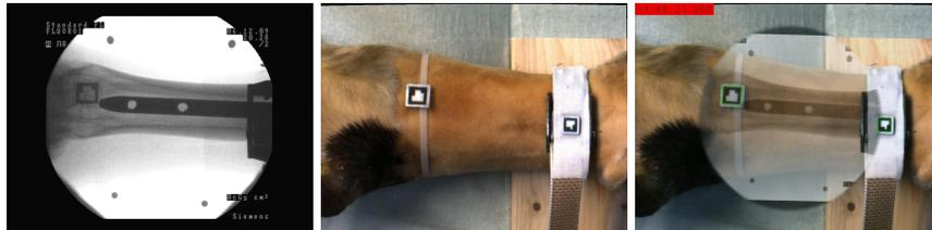
**Fig. 1.** Thanks to a joint construction and calibration, the CamC system register the X-ray image (left) onto the video image (middle) to provide an X-ray and video image overlay (right).
