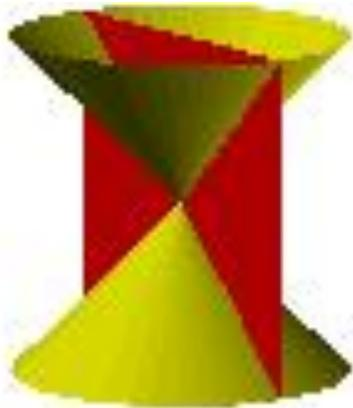
Degenerate conic section: intersecting lines
