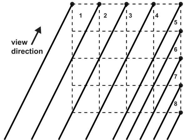
Figure 5: In the special case when the epipolar lines are all parallel, the wedges become parallelograms.
