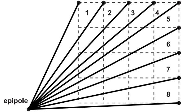
Figure 3: The silhouette image is partitioned into a set of wedges, which are the entries of the Wedge-Cache. In this simple example, the silhouette image is  $4 \times 4$  pixels and there are eight Wedge-Cache entries.
