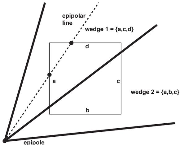
Figure 6: A simple Wedge-Cache example with a square silhouette. The epipolar line is contained in wedge 1, so it need only be compared to edges  $a$ ,  $c$ , and  $d$  for intersection. In fact, the line intersects only edges  $a$  and  $d$ .
