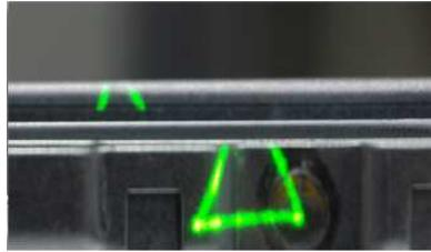
Figure 12: Laser Projection Divided on Multiple Surfaces due to Inadequate Surface
