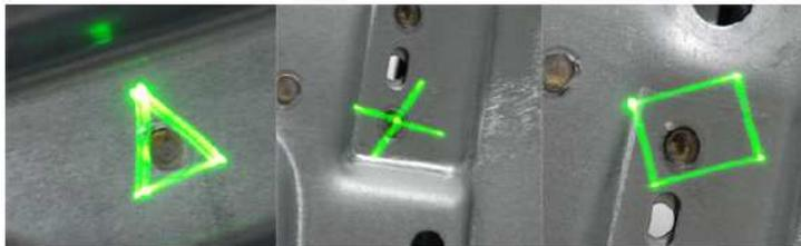
Figure 13: Different Symbols Projected on a Surface by the Laser
