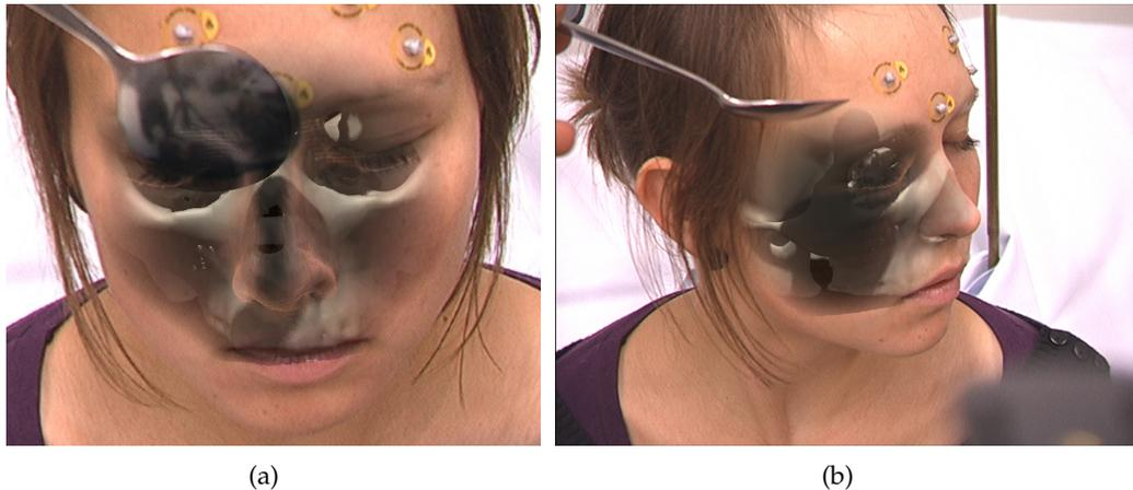
Figure 7.12: Shadow is thrown by a tracked spoon onto the virtual skull.
