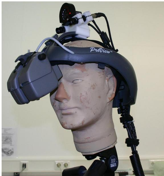
Figure 3.2: HMD with attached color cameras and an infrared camera for inside-out tracking.
