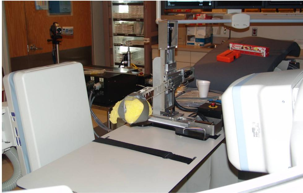
Figure 3.9: Motion platform with attached foam liver centered in C-arm system
