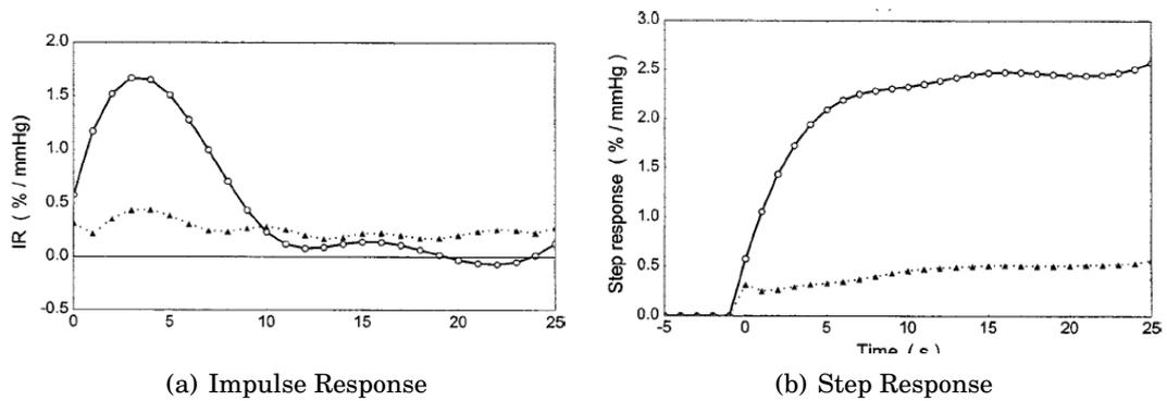
**Figure 3.12** a) Variation in  $V_{MCA}$  impulse response for changes in: (a) Flow regulation time constant; (b)  $CO_2$  reactivity time constant.
