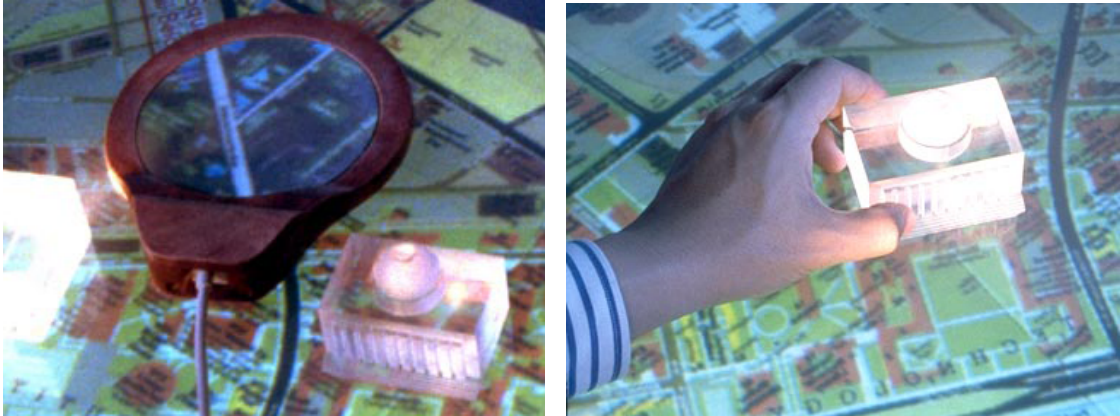
Figure 2.4.: MetaDESK [24]; Left: Great Dome phicon in tangible geospace; Right: a passive lens.
