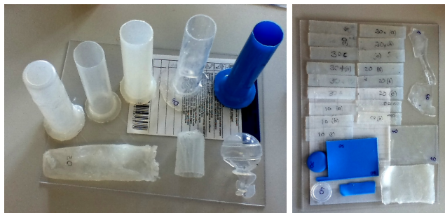
Fig. 2. Vessel phantom prototypes developed for experimental validation of stent deformation. Material samples for each silicone-compound have been tested repeatedly under uni-axial tensile loading.
