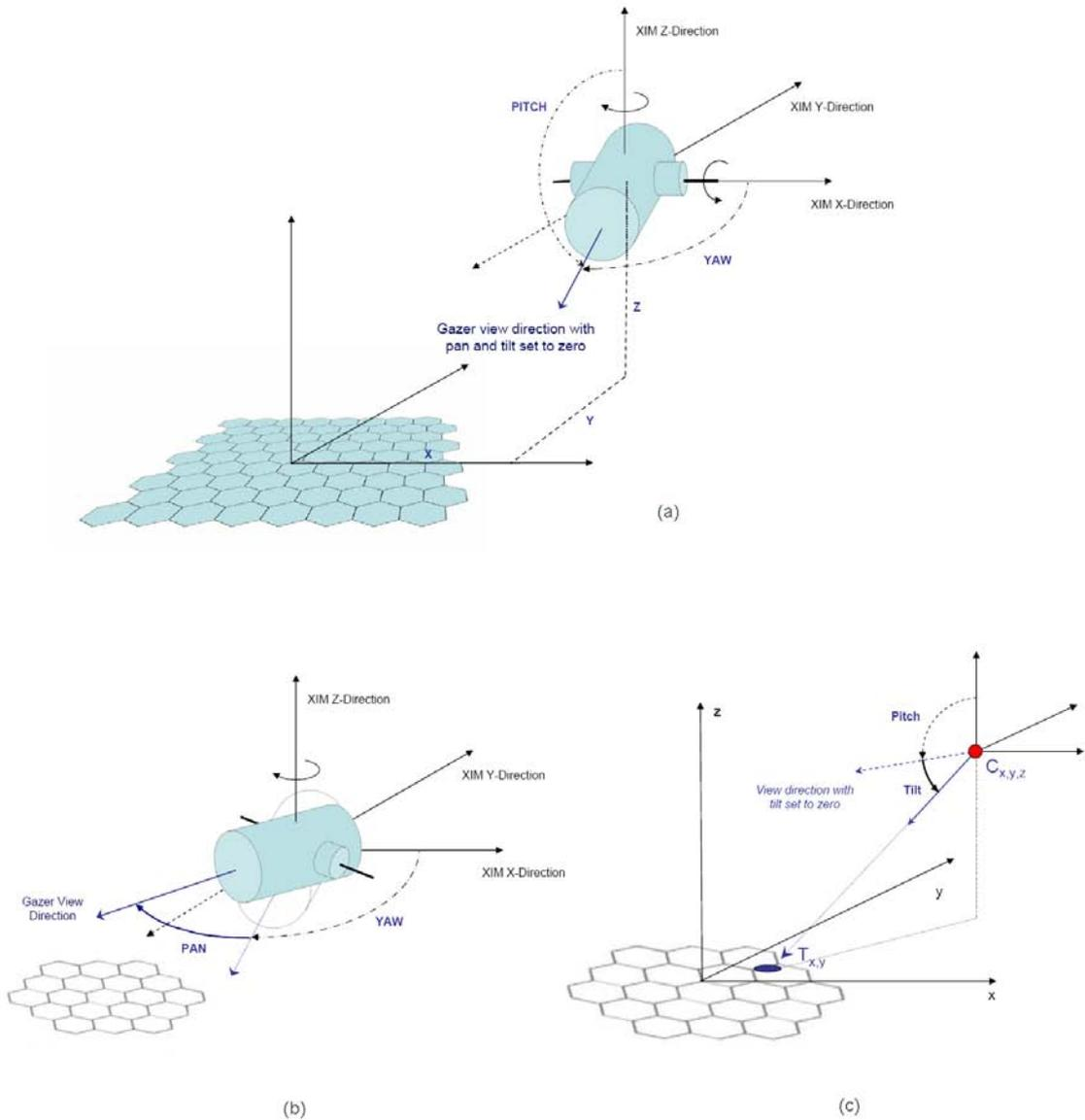
Figure 2.1.: **The pose of a gazer.** Position  $(x, y, z)$  and orientation (yaw, pitch) are defined in relation to the reference coordinate system (a). Yaw and pitch thereby refer to the orientation as the pan and tilt angles are set to zero. The pan describes the gazer's internal rotation around its z-axis (b), while the tilt angle describes the internal rotation around the x-axis and thereby the nod of the camera head (c).
