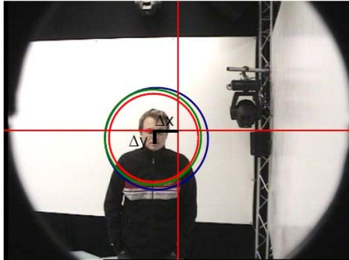
Figure 2.16.: **Deviation in the image after automatic gazer adjustment.** The gazer's orientation was computed from the position of the person seen in the image as signaled by the tracking system.  $\Delta x$  and  $\Delta y$  give a measure of accuracy of the computation. In the perfect case, the person would have to be featured in the very center of the image.
