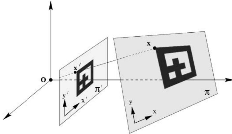
Figure 3.2.: **Homography between marker and image plane.** From a minimum of four point to point correspondences  $\{x_i, x'_i\}$  a projective transformation  $H$  can be computed that maps each point  $x_i$  on the marker plane to its projection  $x'_i$  on the image plane. This relationship can be expressed as  $x'_i = Hx_i$ . *Image adapted from [32]*
