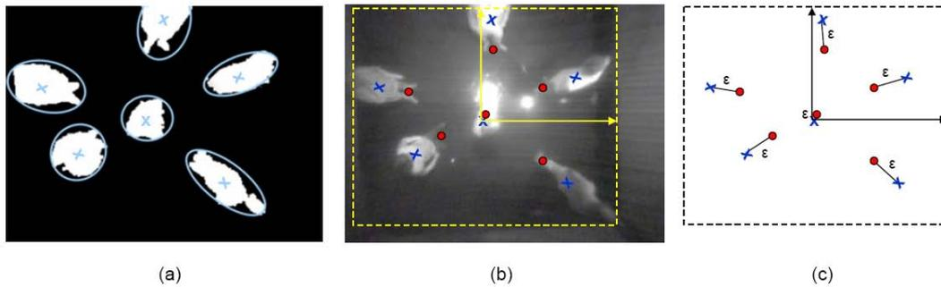
Figure 2.15.: **Perspective distortion in the overhead tracking image.** (a) shows the silhouettes as segmented by the overhead tracking software. As seen in image (b), their centers vary from the positions defined true (the persons positions on the ground floor, marked red in the image). This perspective error  $\epsilon$  increases as the person moves further away from the center of projection (c).
