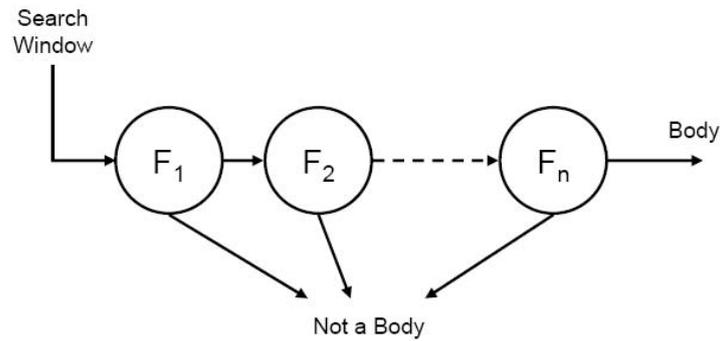
Figure 2.4.: **Object detection cascade of classifiers where rejection can happen at every stage.** Image adapted from [16]
