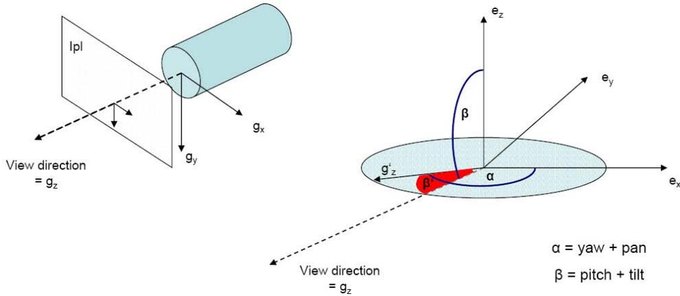
Figure 3.8.: **Model for the retrieval of the yaw and pitch angles from the rotation matrix.**
