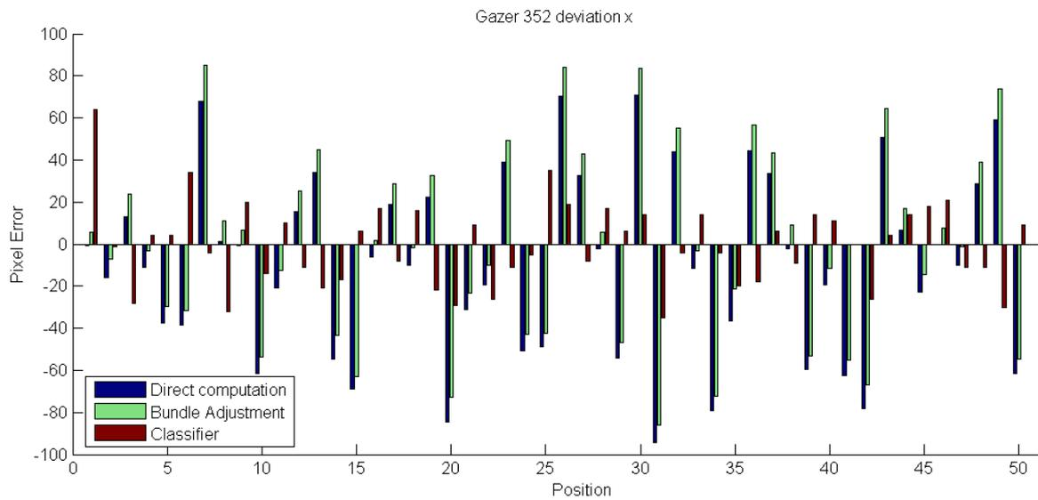
Figure 3.16.: Accuracy of gazer 352 in the person tracking experiment under the different calibrations.
