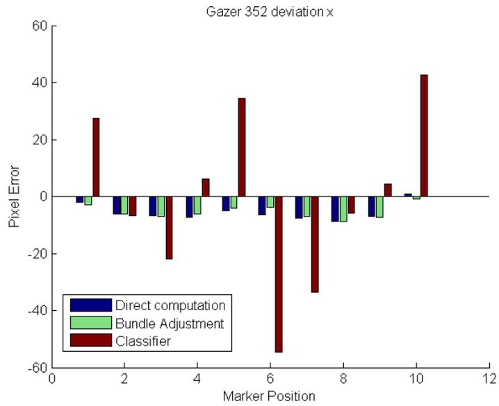
Figure 3.22.: Accuracy of gazer 352 in the marker reprojection experiment under the different configurations.
