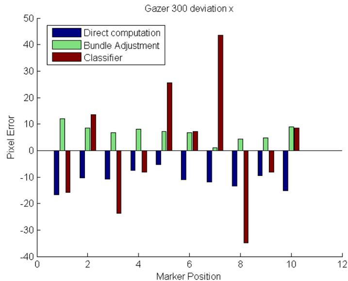
Figure 3.21.: Accuracy of gazer 300 in the marker reprojection experiment under the different configurations.
