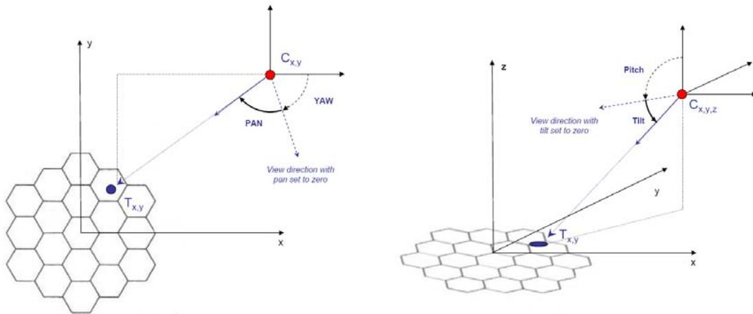
Figure 1.7.: The model for the computation of the pan and tilt angles for a gazer to look at a specific position  $T$ . Mandatory are, along with the tracking data  $T$ , the gazer's position  $C$  and orientation in 3D space, furthermore referred to as *yaw* and *pitch*.
