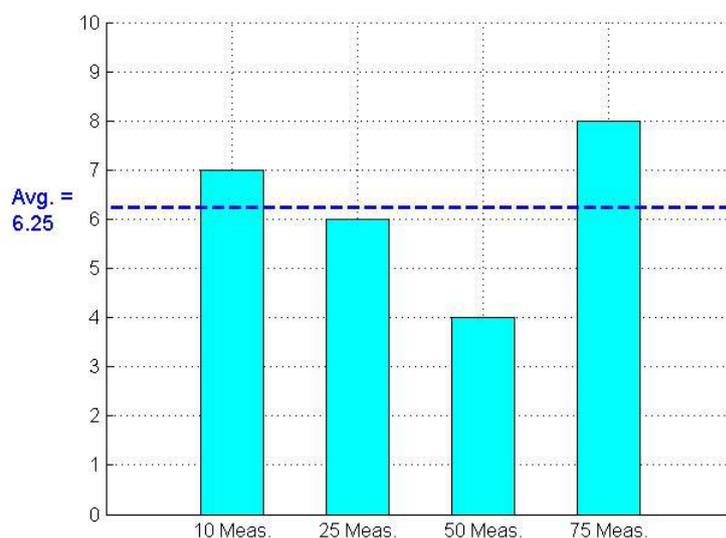
Figure 2.12.: **Steps necessary for the LMA to reach convergence for measurement sets of different size.** After an average of 6.25 steps, the variation in the Sum of Squared Differences was below a limit of 0.1 in each step.
