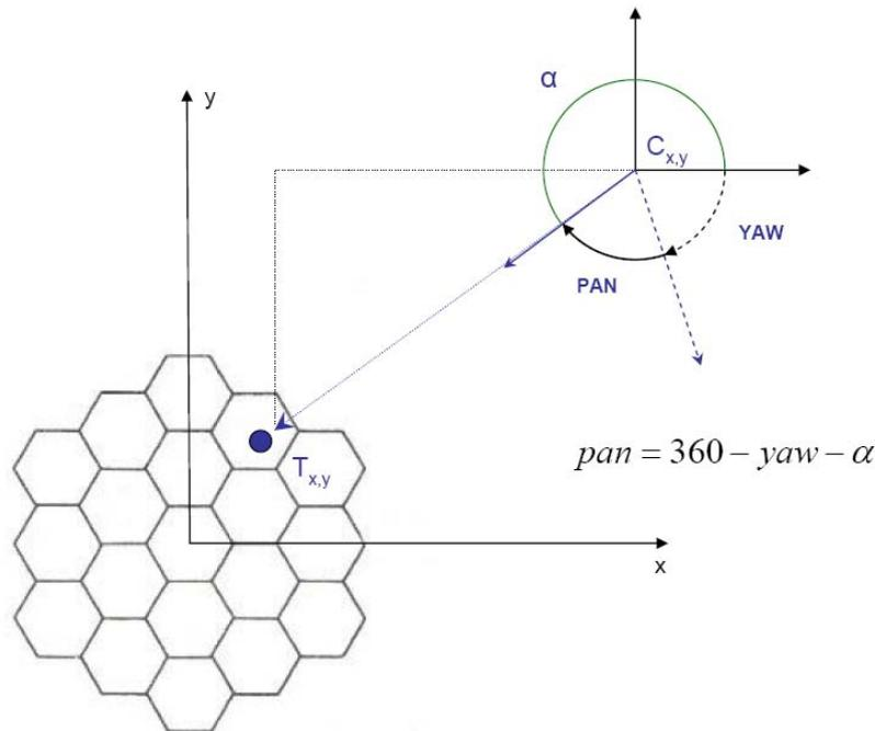
Figure 2.5.: **Computational model for the pan angle.** The angle  $\alpha$  can be computed trigonometrically. The pan angle can then be determined by subtracting  $\alpha$  and the yaw of the gazer from the full euclidean unit circle.
