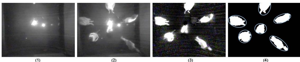
Figure 1.4.: **The image processing pipeline of the 3D tracking system AnTS.** The background image (1) is subtracted from the current camera image (2) to reveal all objects that set themselves off from the floor (3). (4) shows the image after processing, whereby each ellipse indicates the boundaries of an object.
