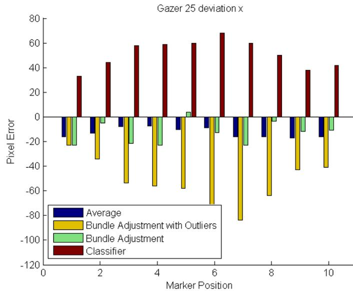
Figure 3.20.: Accuracy of gazer 25 in the marker reprojection experiment under the different configurations.
