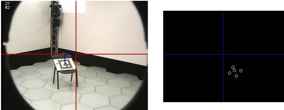
Figure 3.18.: **Setup for the comparison on basis of a reprojected marker.** We want to determine the deviation between marker and image center (left). The pose of the marker as computed from the overhead camera image (right) yields the exact position of the marker in the space.
