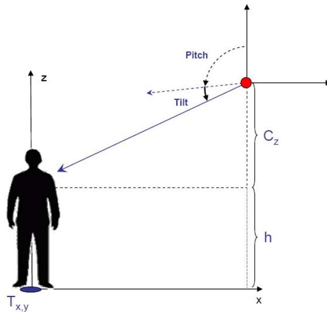
Figure 2.7.: **Significance of the estimated gazer height.** The measured tilt angles, and thus the estimated height of the gazer  $C_z$ , relate to the person's upper body height  $h$ .
