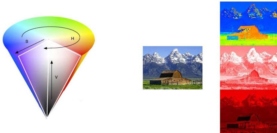
Figure 4.4.: **Conical representation of the HSV color space (left) and an image along with its h, s and v components (right).**
