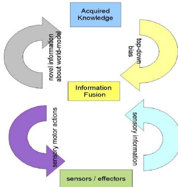
Figure 1.5.: **Top-down modulation of bottom-up sensory information as implemented in the MMT.** The individual sensors deliver data to the data fuser. The data fusion process is modulated by the input from the world-model. The result of the data fusion is then used to update the world-model and also to actively deploy sensors and effectors. *Image adapted from [39]*
