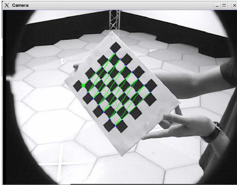
Figure 3.7.: **Intrinsic camera calibration using the Ubitrack chessboard calibration pattern.**
