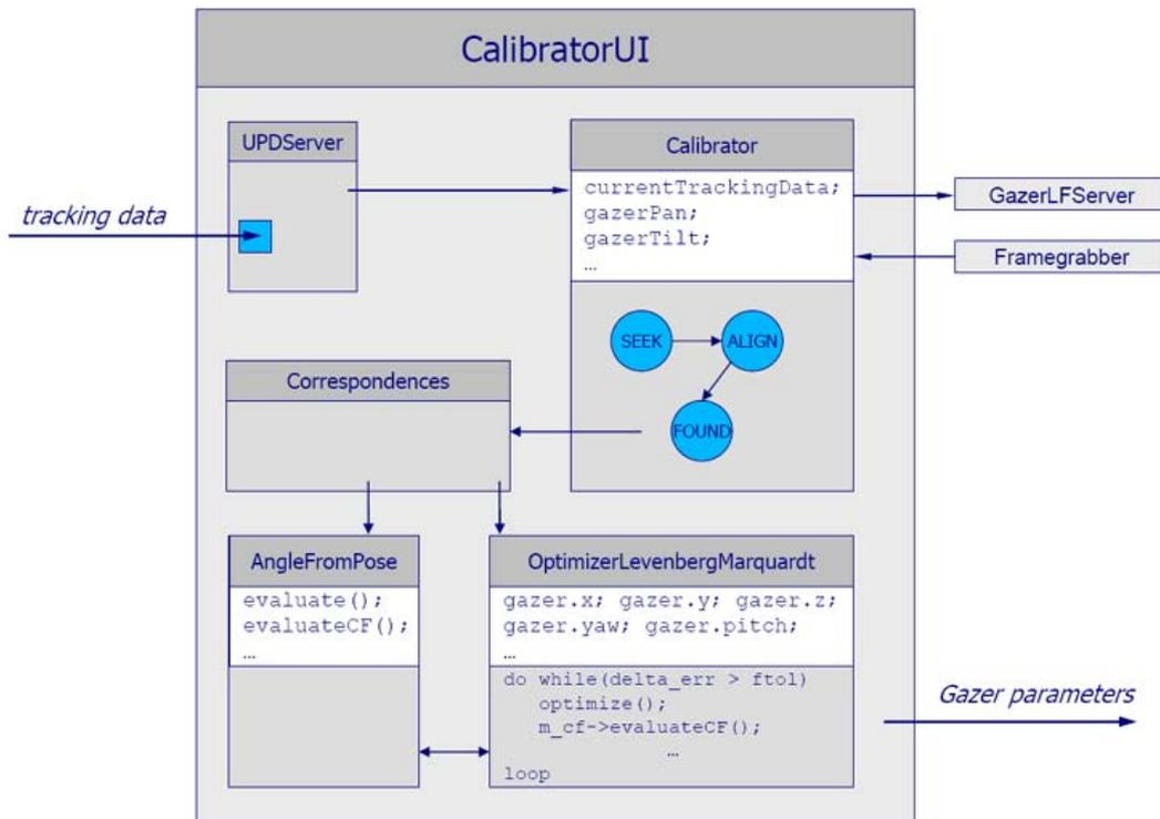
Figure 2.8.: **Overview of the system design for the classifier approach.** The core of the application is a `Calibrator` class that seeks the correspondences. Once enough correspondences have been found, the extrinsic gazer parameters are optimized by a Levenberg-Marquard Optimizer.
