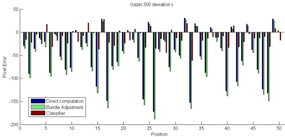
Figure 3.15.: Accuracy of gazer 300 in the person tracking experiment under the different calibrations.
