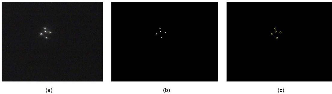
Figure 3.4.: **Processing of the infrared camera image.** The infrared LEDs attached to the marker can be clearly extinguished in the image of the infrared camera (a). By simple thresholding (b) and region detection the marker vertices can be identified (c).
