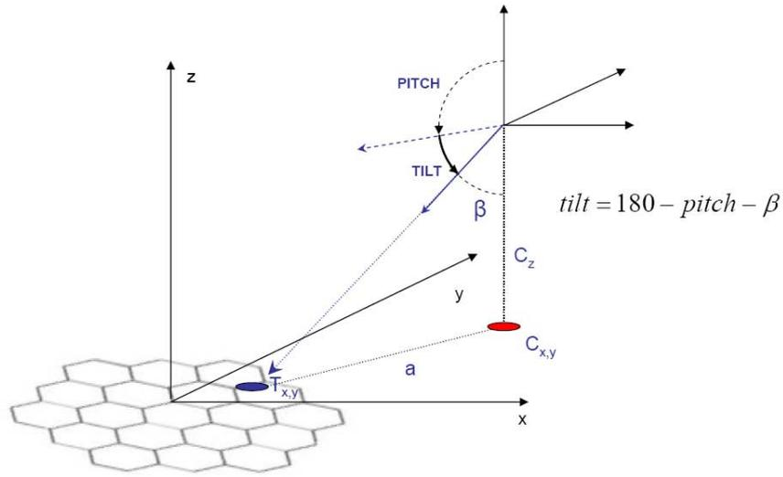
Figure 2.6.: **Computational model for the tilt angle.** The angle  $\beta$  can be computed trigonometrically. The tilt angle can then be determined by subtracting  $\beta$  and the pitch of the gazer from half the unit circle.
