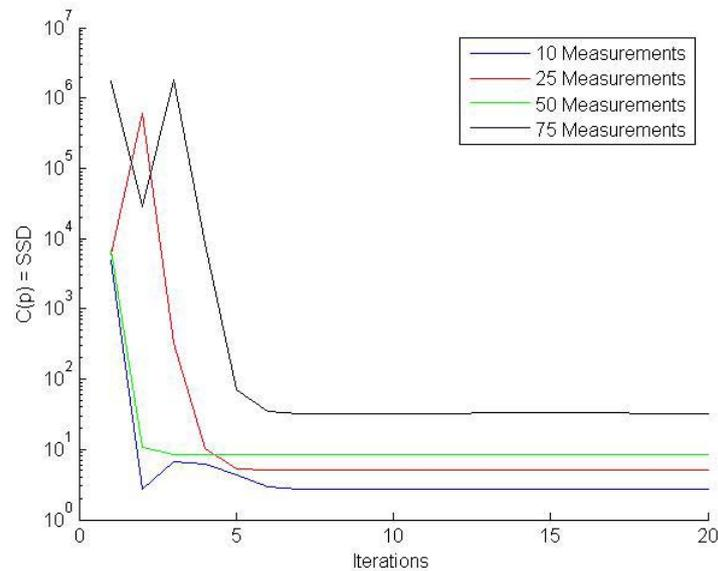
Figure 2.11.: **Convergence of the Levenberg-Marquard Optimizer.** The algorithm was tested for input measurement vectors of different size and proved to converge toward a final parameter vector within few steps. Thereafter the Sum of Squared Differences changed only slightly before the algorithm terminated.
