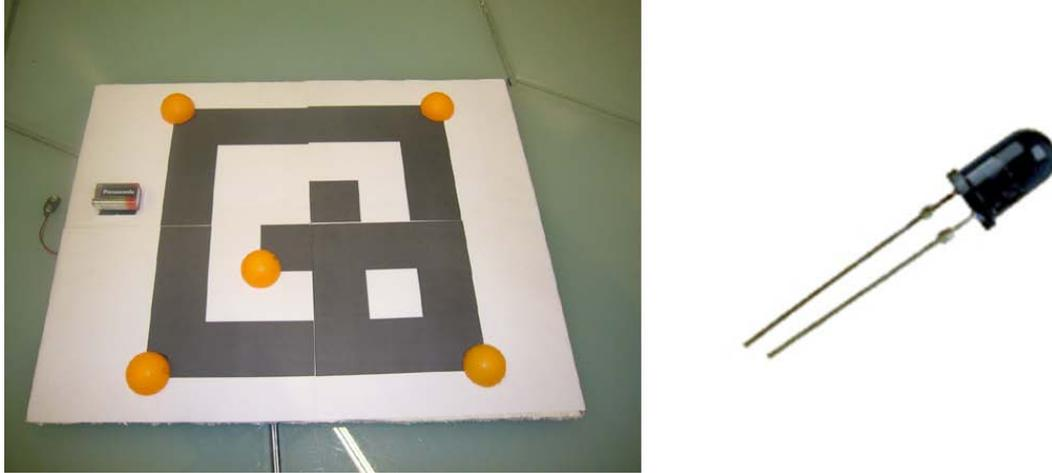
Figure 3.3.: **The interactive marker used for the control experiment.** Five infrared light emitting LEDs were installed at well defined vertices of the marker to make them visible to the infrared overhead camera. To avoid artifacts due to diffusion, the LEDs were covered with semi-transparent hemispheres.
