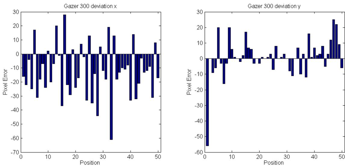
Figure 2.19.: Accuracy of gazer 300 in the test scenario.
