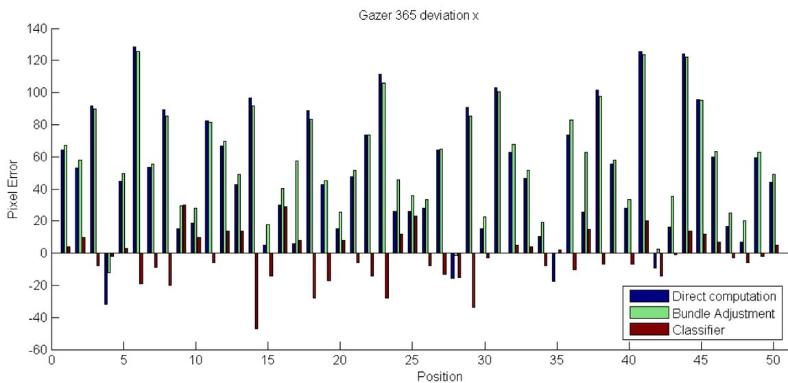
Figure 3.17.: Accuracy of gazer 365 in the person tracking experiment under the different calibrations.
