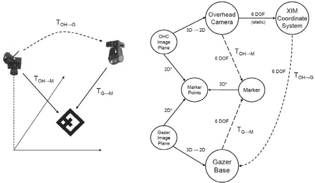
Figure 3.1.: **Setup for the control experiment.** The transformation  $T_{OH \rightarrow G}$  between the overhead camera and the gazer is estimated by concatenating the transformations between overhead camera and marker and between gazer and marker.
