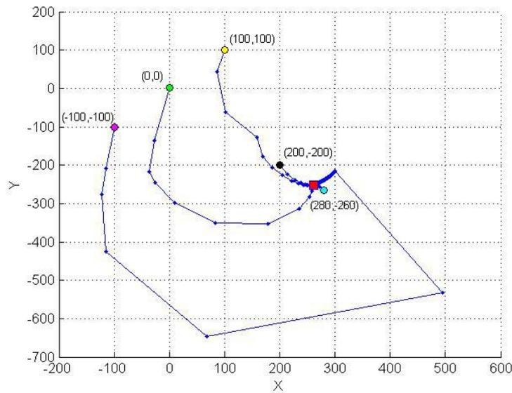
Figure 2.13.: **Optimization path of the gazer position.** Different starting parameters were provided to the LMA as an input. Independent of their choice, the algorithm terminated with a well-defined output (marked as the red square).
