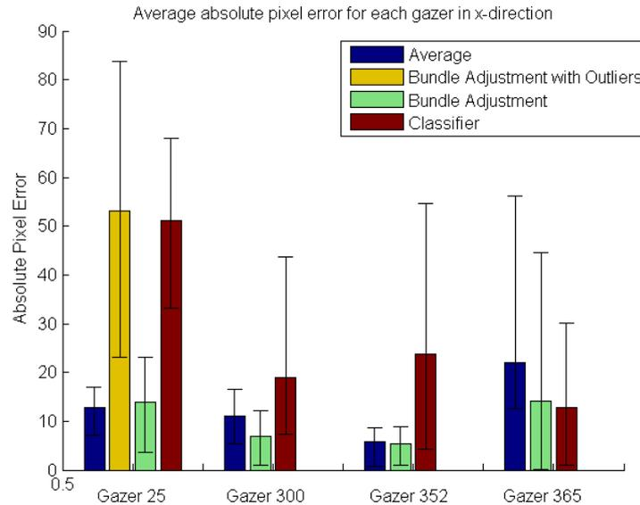
Figure 3.19.: Average absolute deviations of the marker from the image center for the different calibrations of the gazers.
