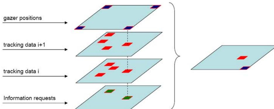
Figure 4.2.: Creation of a saliency map from a set of input sources.
