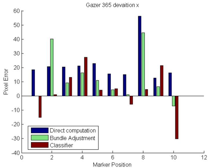
Figure 3.23.: Accuracy of gazer 365 in the marker reprojection experiment under the different configurations.
