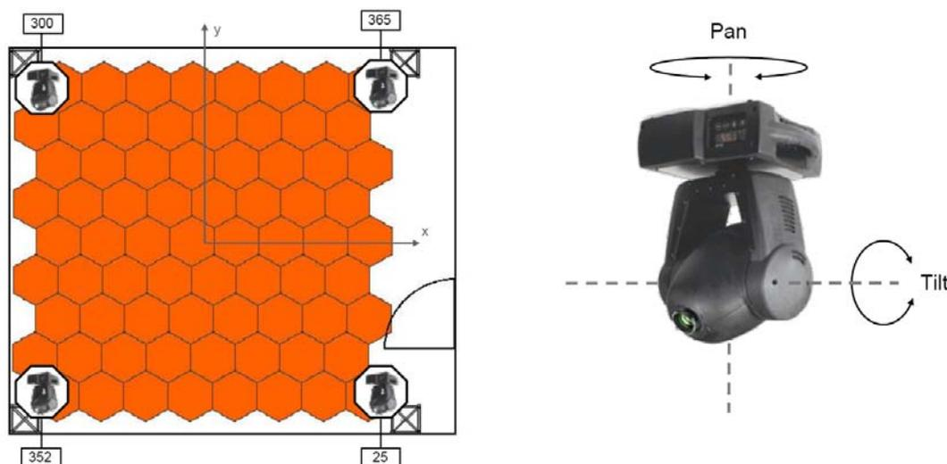
Figure 1.6.: **Gazers in the XIM.** The individually controllable pan and tilt cameras, the "gazers" (right figure), are mounted to the rig on head height in the four corners of the XIM (left figure).
