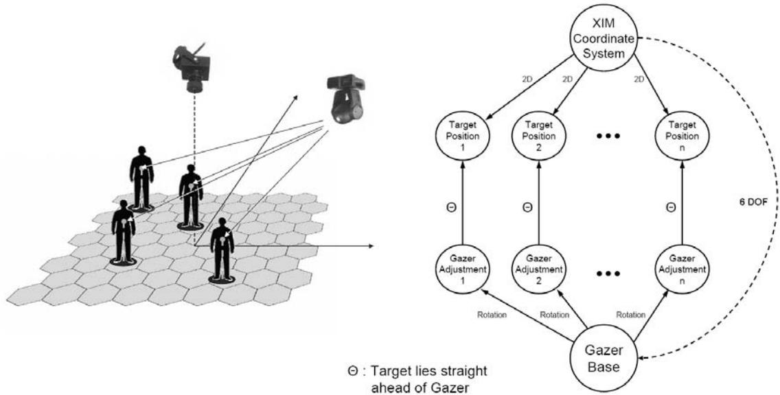
Figure 2.2.: Conceptual setup for the classifier approach to estimate the extrinsic pose of a gazer.
