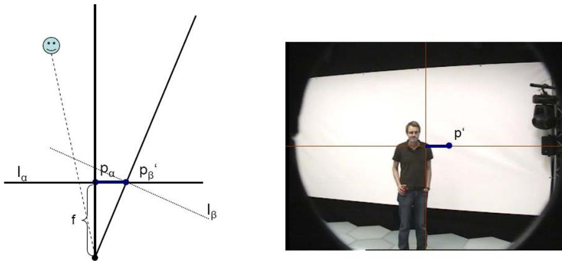
Figure 3.12.: Computation of the shift between two images  $I_\alpha$  and  $I_\beta$ .
