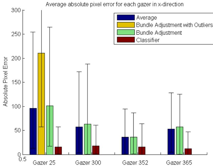
Figure 3.13.: Average absolute deviations in x-direction for the different calibrations of the gazers.
