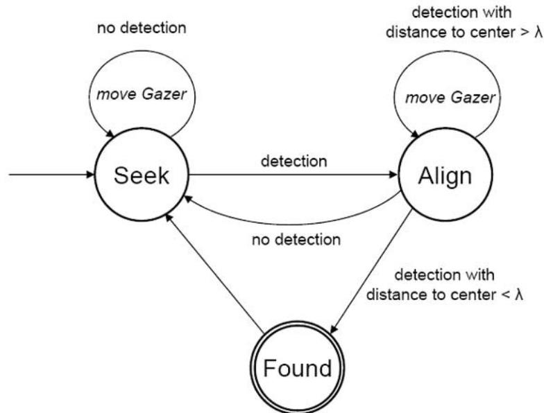
Figure 2.9.: **State chart for the Calibrator.** In the *Seek* state the gazer is iteratively rotated around both axes while the classifier scans the camera image to detect the person. If a person was detected the application switches to the *Align* state and tries to adjust the gazer so that the person is located right in the center of the image.
