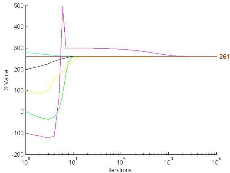
Figure 2.14.: **Convergence of the LMA for different starting parameters.** Regardless of the initial values, the different parameters (shown here is the x value) quickly approached their final value.
