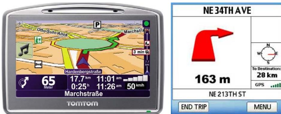
(a) Map-based navigation system (Courtesy of TomTom) (b) Symbolic turn-by-turn navigation system (Courtesy of Telenav)
