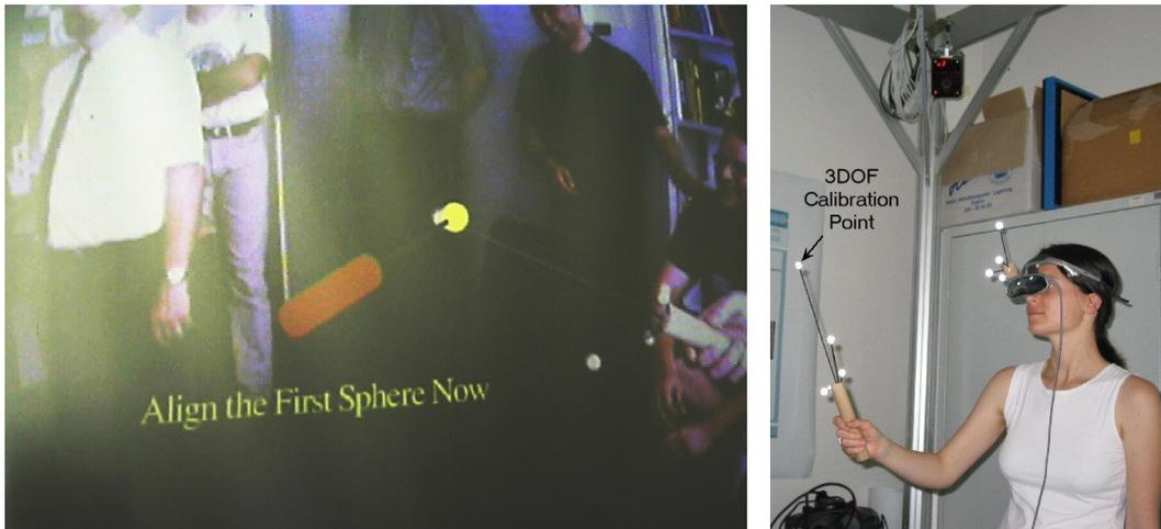
Figure 3.6: HMD calibration with a pointing device
