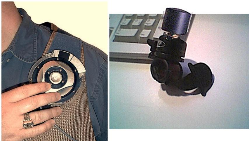
Figure 11.4: Left: CMU VuMan dial device; Right: mockup of custom potentiometer device
