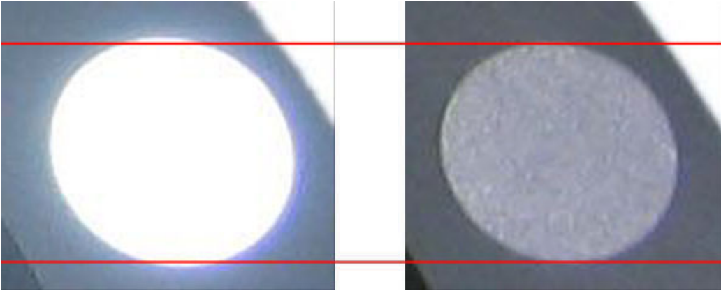
Figure 34: Images showing the same retro-reflective fiducial photographed with and without a flash. The red line is aligned with the top and the bottom of the correctly illuminated fiducial on the right. Bright regions in an image appear larger than their counterparts due to overexposure. This effect is called overshining.
