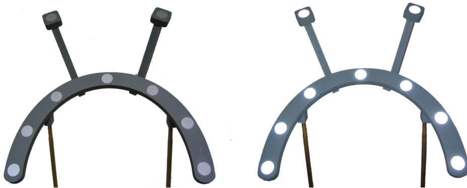
Figure 14: The fiducials are glued on plastic frame as a set of fiducials. The left photo has been taken without a flash and the right one with a flash.
