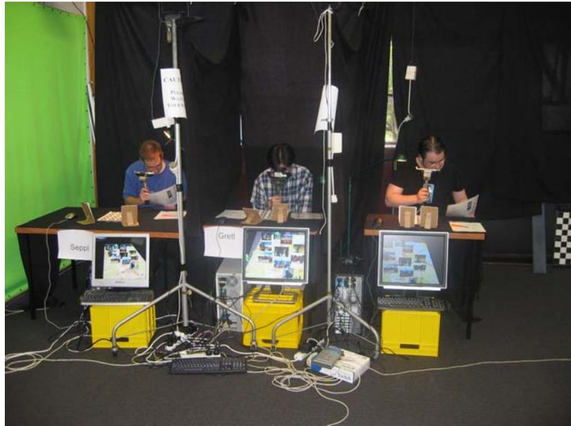
**Figure 5.2:** Photograph of the set-up: three users collaborating with the handheld displays and their view of the scene in the monitors
