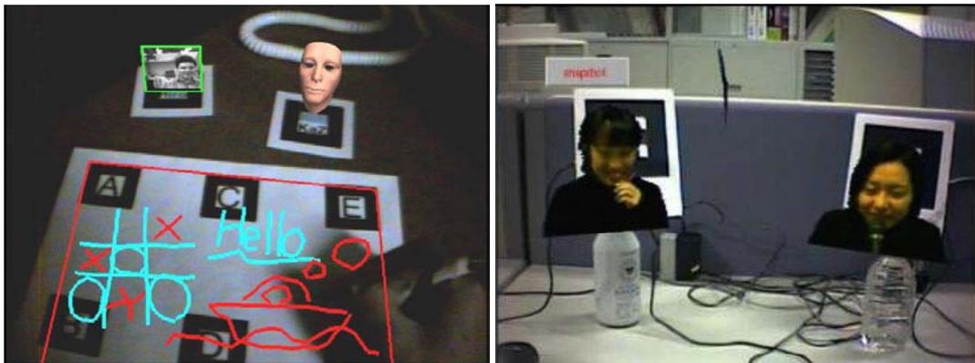
**Figure 3.6:** a) typical setup of the AR videoconferencing application with the virtual shared white-board b) background elimination of the remote users (taken from [KBMT01])
