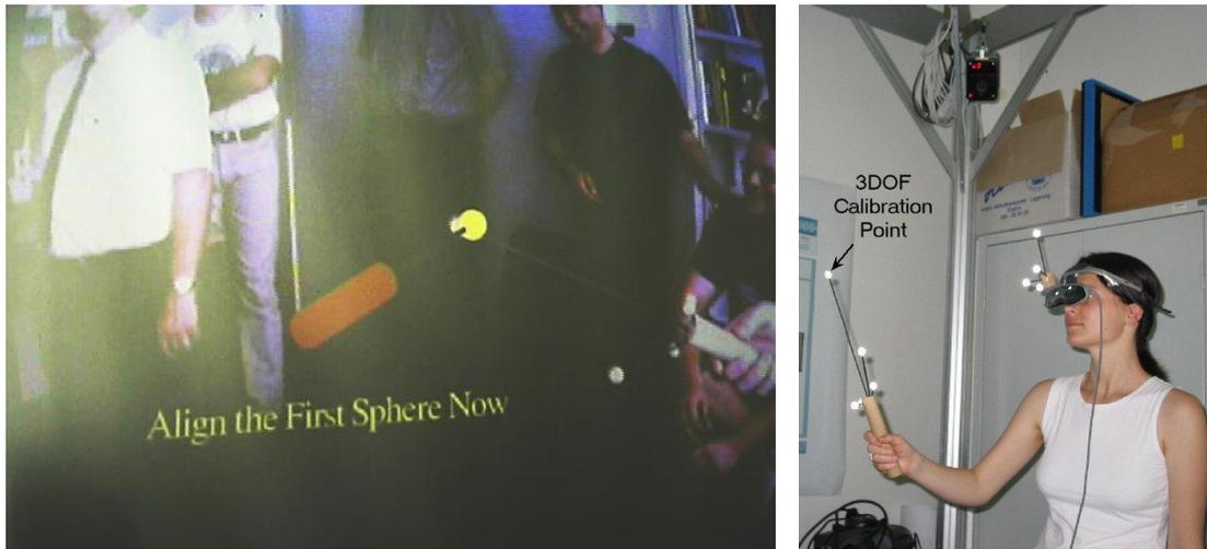
Figure 2.6: HMD calibration with a pointing device
