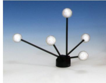
Figure 2.2: Infrared Marker
