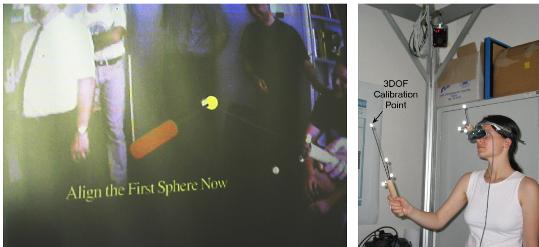
Figure 3.1: HMD calibration with a pointing device
